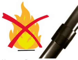
No open flames when cementing. No smoking.
