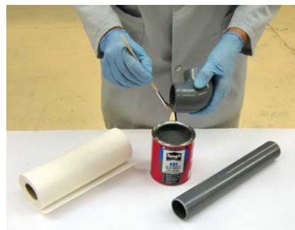
Applying the cement
